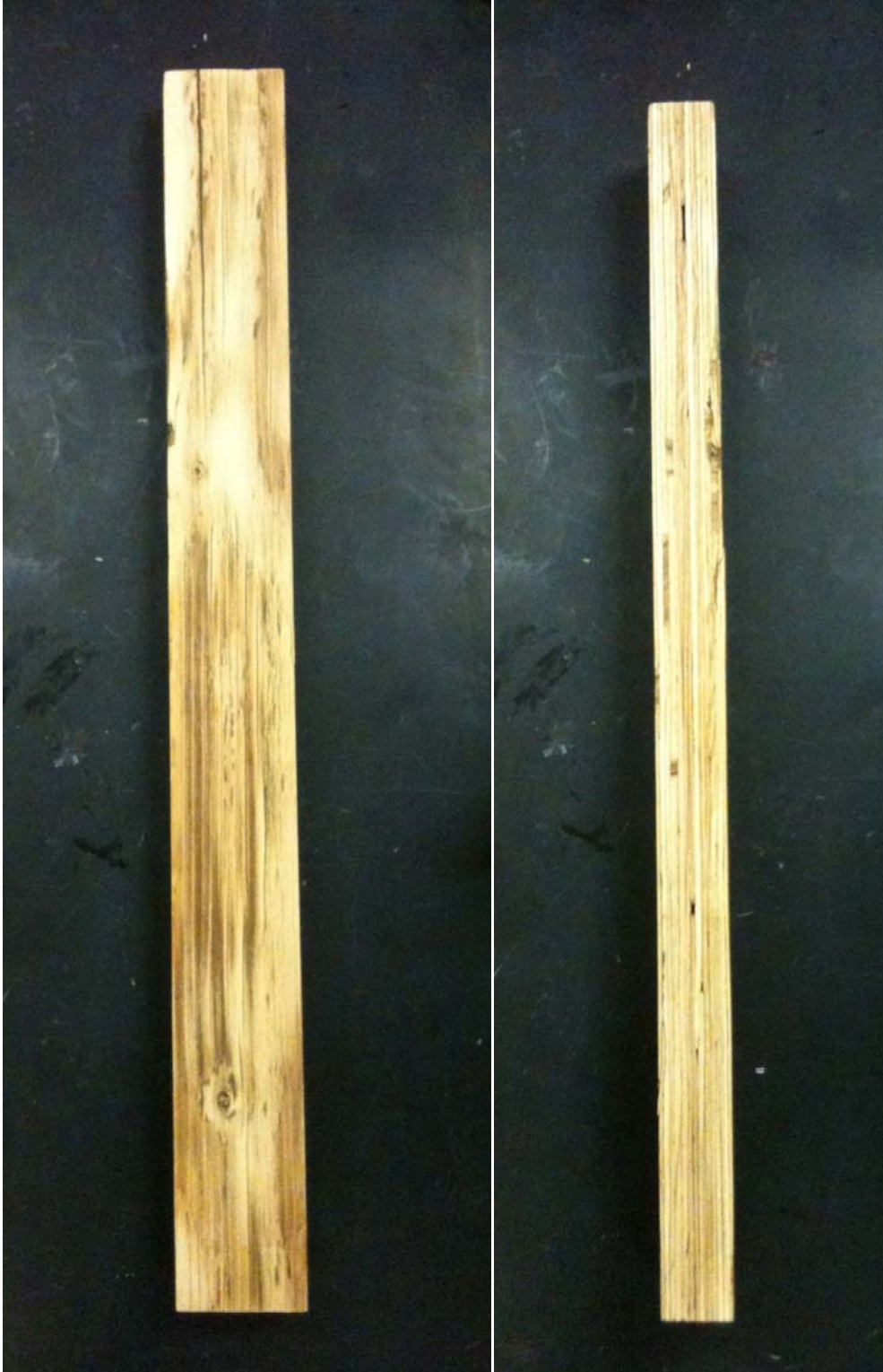
Figure 1. Typical untreated ILevels Microlam 1.9E Douglas-fir LVL. These samples were received by LSU WDL milled down to the actual testing size of 1 3/4" x 3" x 30".
